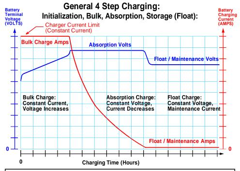
**Step 1) Initialization:** Red Light On or Red Light Flashing: Monitor Circuit verifies appropriate battery voltage levels and good electrical continuity between the battery and the charger DC output.
