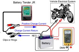
Note: After the battery voltage reaches 14.4 volts, the Battery Tender JR will go into the float / maintenance, storage mode.
